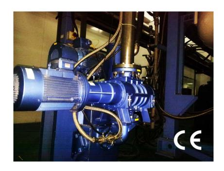
Custom made ERA900M/EMBD540 is widely used on the multi-silicon crystal growing furnaces
