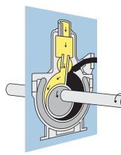
Depending on your application and what vacuum level you need to attain, Kinney Pumps are available in either single-stage or two-stage design. The two-stage pumps will achieve a lower vacuum level due to the two piston chambers which are arranged in series with a connecting channel.
