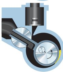
These three facts, the oil seal, the filling of the clearance volume, and no contact between piston and wall, are what give the rotary piston pump its low blank off, high pumping speeds at low pressures and great durability.
